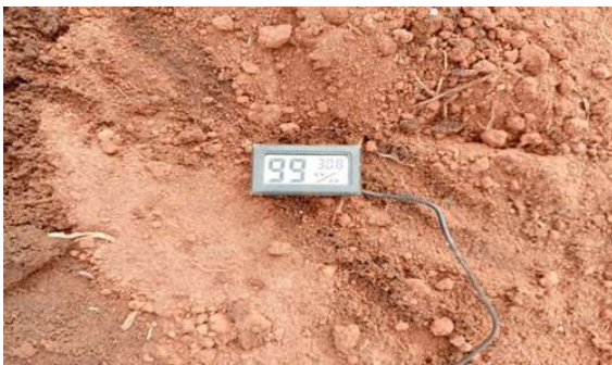
Figure 5. Appearance of excavated holes: closed hole with sensor installed
