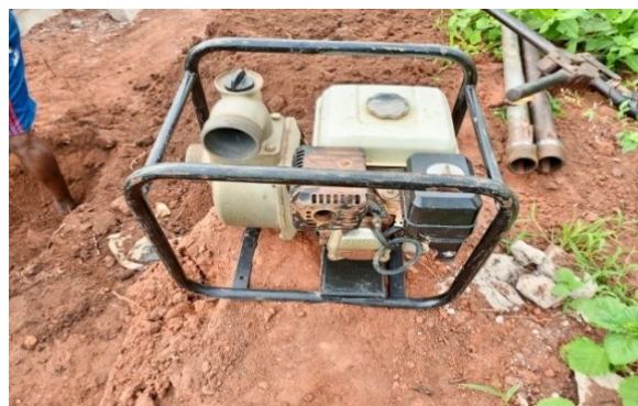
Figure 2. Manual drilling equipment: motor pump
