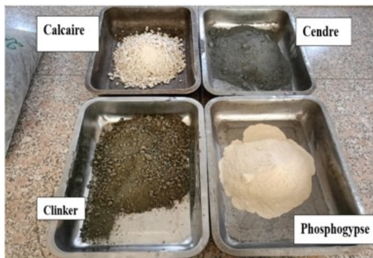
Figure 2. Raw materials used for cement production in the laboratory
