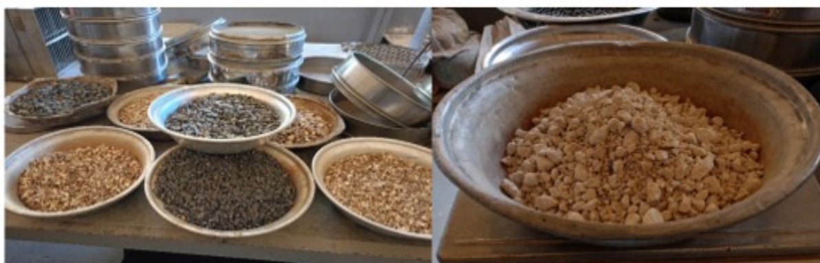
Figure 4. Aggregates used in hydraulic concrete formulations
