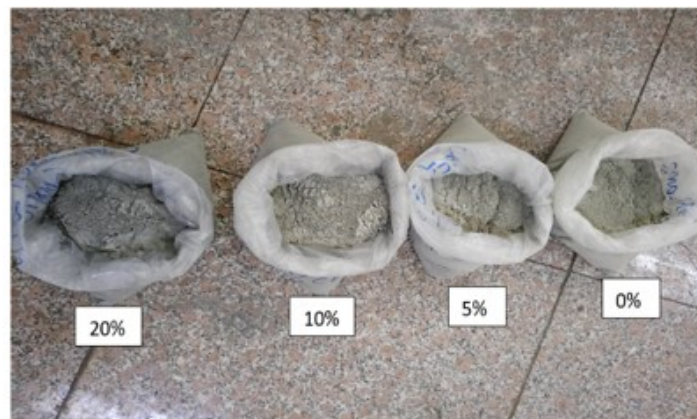
Figure 3. Cement obtained after grinding and sieving through a 1 mm diameter sieve for different ash contents (0%, 5%, 10%, 20% respectively from lightest to darkest) [4] and [5]
