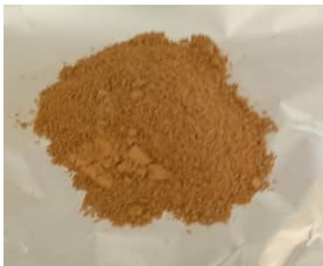
Figure 2. Physical aspect of Sinématiali alum sludge dried at 110°C
