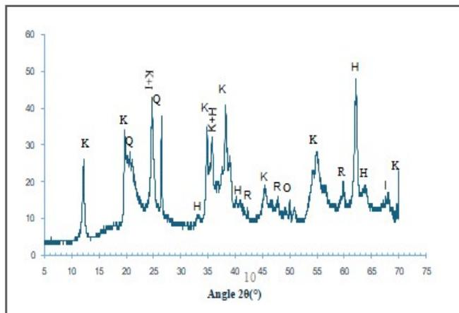
Figure 3. XRD pattern of the studied alum sludge
