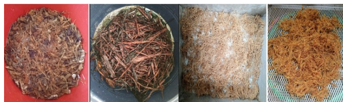
Figure 4. The fibers and residues of Borassus wood treated with soda
