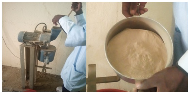
Figure 2. Electric machine for grinding residues into powder
