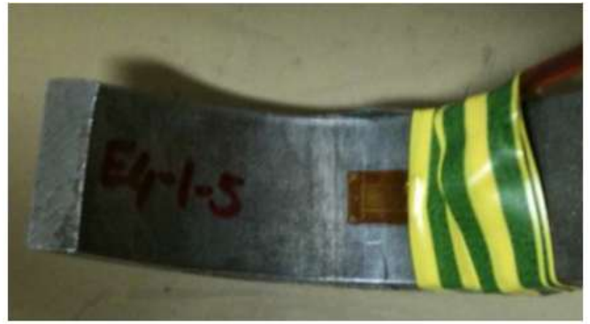
Figure 3. A specimen after strain gauge installation
