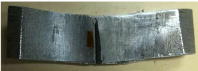
Figure 8 racked specimen after fatigue test
