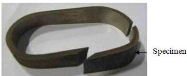
Figure 2. A specimen cut from a section of the rotor
