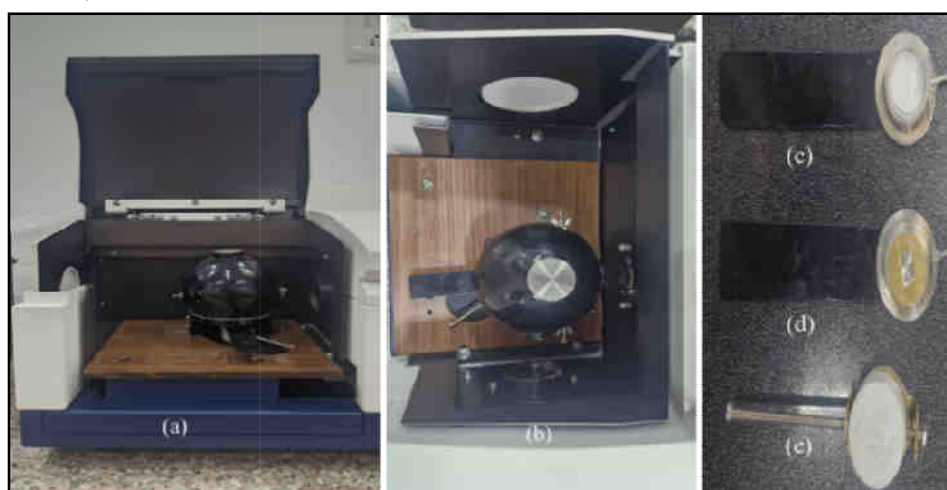
Figure 1. Integrating sphere mounted inside the sample chamber of the Hitachi F-7000 fluorescence spectrophotometer (a) front view, (b) top view, (c) liquid sample holder, (d) solid sample holder and (e) spring arrangement to hold sample holder in the hole at the bottom of the Integrating sphere
