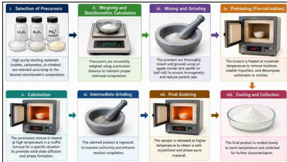
Figure 2: Steps involved in the synthesis of the phosphors by solid state diffusion method
