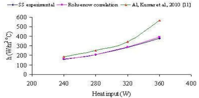
**Fig. 2: Variation in convective heat transfer coefficient with heat inputs**
