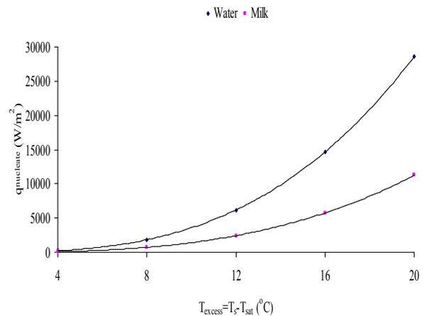
**Fig. 3: Variation in heat flux with heat inputs**
