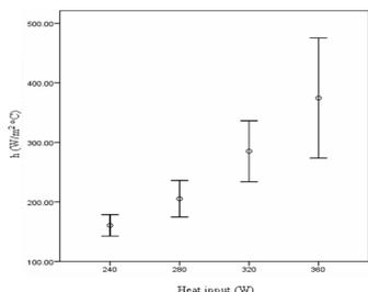
Fig. 4: Error bars for convective heat transfer coefficients
