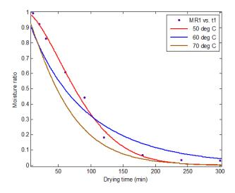
Fig. 1. Variation of moisture ratio with time at different drying temperatures (using Page model)
