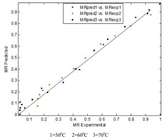
Fig. 5. Comparison of experimental and predicted moisture ratio with time at different temperatures using Page model
