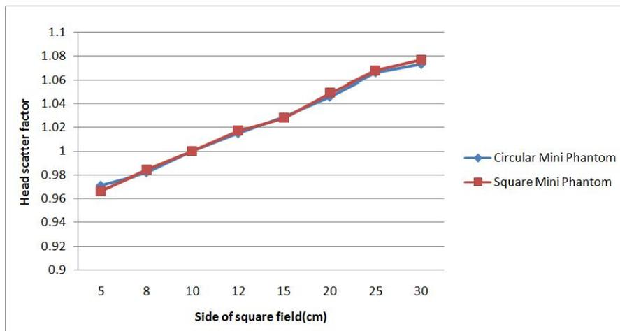
Fig 3. Comparison of different shape of mini-phantoms on Sc measurement
