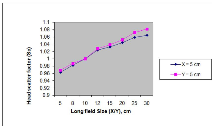
Fig 4. Collimator exchange effect Phoenix-147 Cobalt Unit
